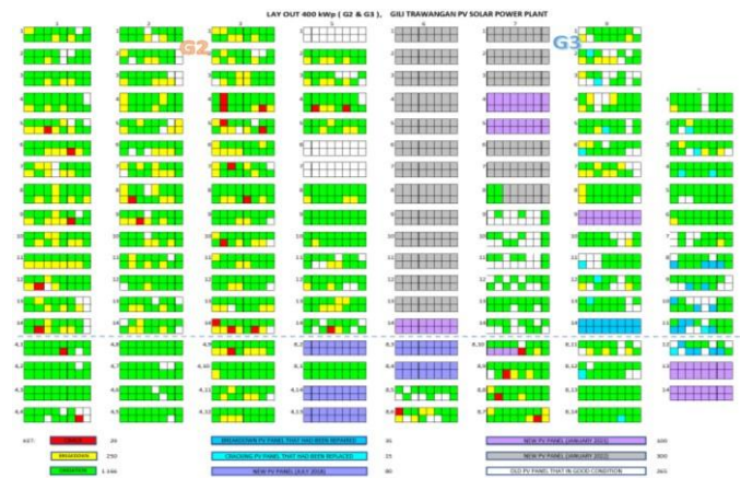
Fig. 2. PV Array and Module Failure Mapping of Gili Trawangan PV Power Plant
